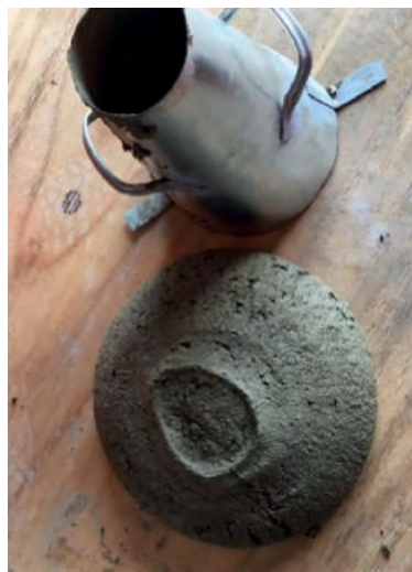
Wi Mortar at 100mm slump
